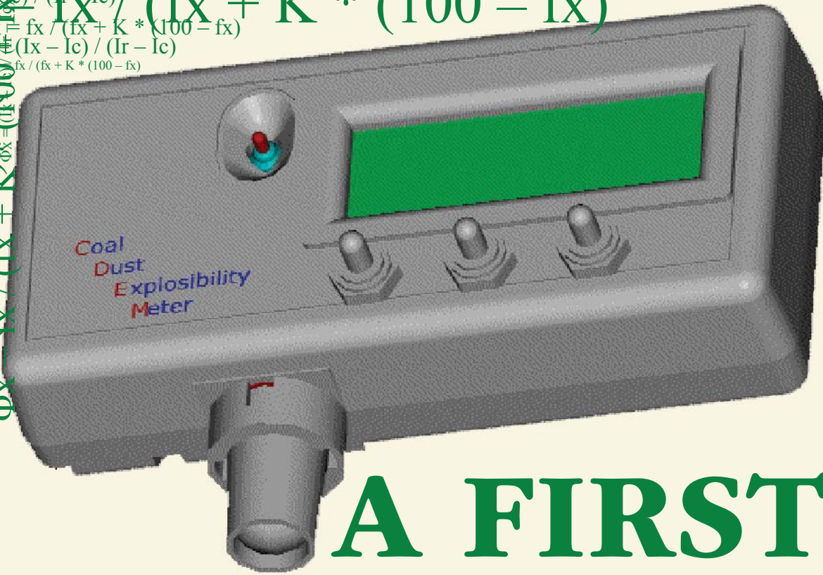
The CDEM—the handiwork of Geneva engineering faculty and students in conjunction with the National Institute of Occupational Safety and Health—enhances mine safety by testing for dust-explosion hazards on site.
